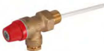
Temperature & pressure relief valve** 1/2" NPT x 15mm (7 bar/90°C)
