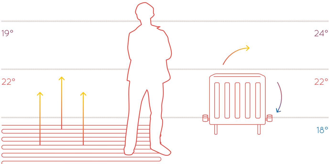
Underfloor heating provides an ideal temperature profile due to radiant heat.
