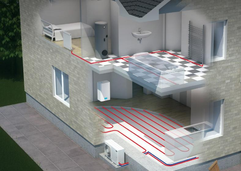
How do Enviroair Air Source Heat Pumps Work? Put simply, the Enviroair air source heat pump works by using a refrigeration process to transform low-grade energy from the outside air into high-grade energy.
